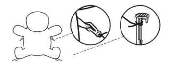
For inflatables under 9-feet tall, install at least three upper tie downs. For inflatables over 10-feet tall, you will need to install four or more upper tie downs, depending on the inflatable.
