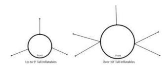
To properly secure your inflatable, install the upper tie downs according to the above graphic. Note that two of the side tie downs must angle forward by at least 30 degrees. Adjust stakes as needed to assure that the inflatable is fully upright and positioned correctly. When the inflatable is correctly positioned and all stakes have been placed, push all of the stakes fully into the ground.
